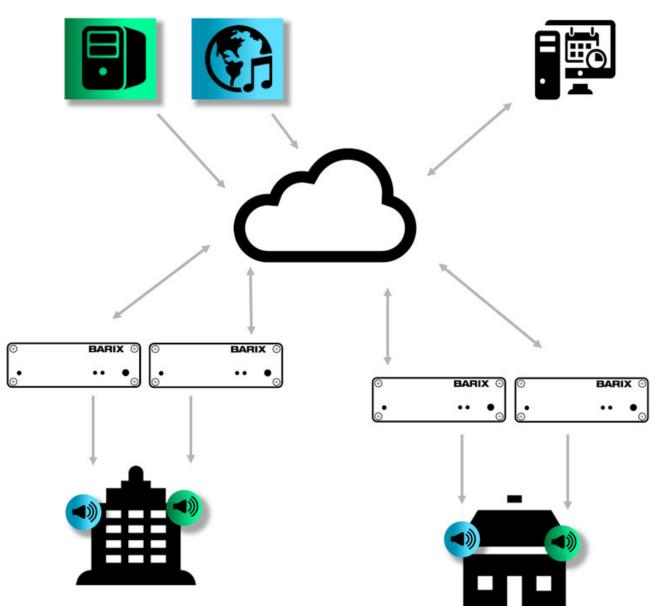
SoundScape is a complete solution to manage and distribute audio over IP networks. With SoundScape, service providers now have a single, centralized solution for content delivery and network-wide monitoring and management, instead of requiring different platforms.
